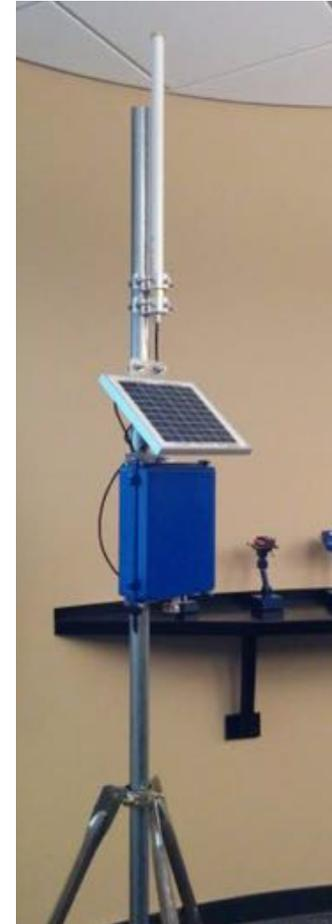
***The Gateway collects the data from the sensors and push it to the Cloud***
